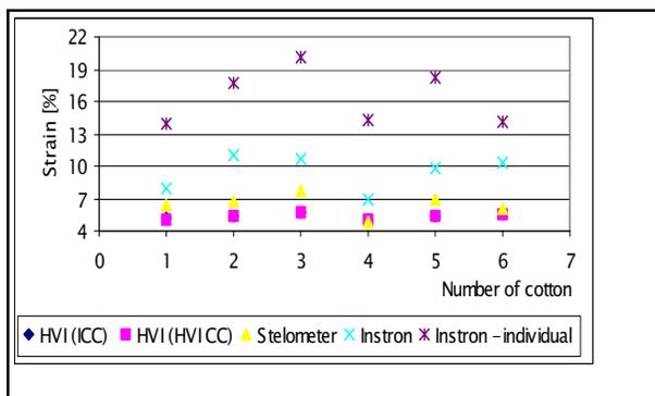
Fig.4b The cotton breaking strain according to the different measurement methods.
