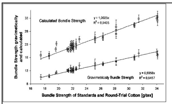
Fig. 7. Measured and Calculated Bundle Strength
