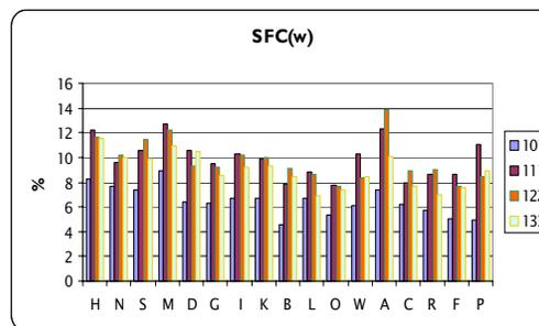
Fig.14. SFC from AFIS reproducibility according to Polish Round-test
