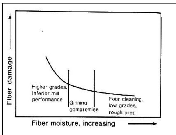
Fig. 2: The acceptable moisture content of cotton being ginned is a compromise between grade level and fiber damage (From Cotton Ginners Handbook, no 503).
