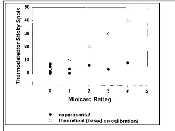
Fig.11. Thermodetector vs. Minicard Ratings for a Series of Whitefly Honeydew Contaminated Samples
