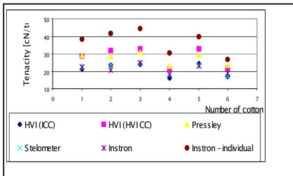
Fig.4a The cotton strength according to the different measurement methods.
