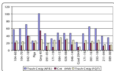
Fig. 15 b. The number of trash particles in cotton according to the optoelectronic measurements
