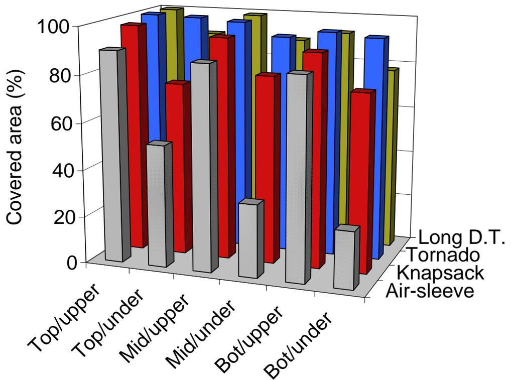
**Figure 5: The droplet density found with UV tracer for the tractor mounted and for the Drop-tube knapsack sprayer.**
