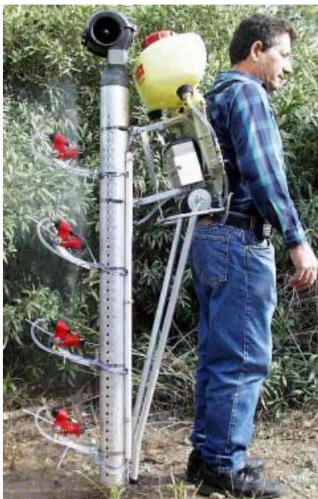
A 12 Volts rechargeable battery is providing the power to the atomizers and to a blower mounted at the top of the sprayer. The blower blows the air through a perforated tube with many small outlets along the two sides. The streams form air curtains directed toward the row on both sides of the sprayer. The spray droplets created by the atomizers are released and mixed in the air curtains, which carry them until deposition on the cotton canopy. [1998 report, p. 122].
