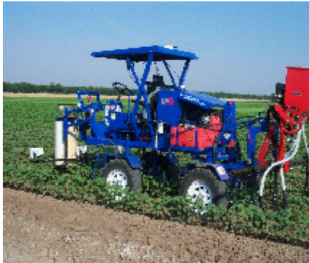
Figure 2. 4WD research vehicle with IR, GPS, variable rate fertilizer application and insect vacuuming system.
