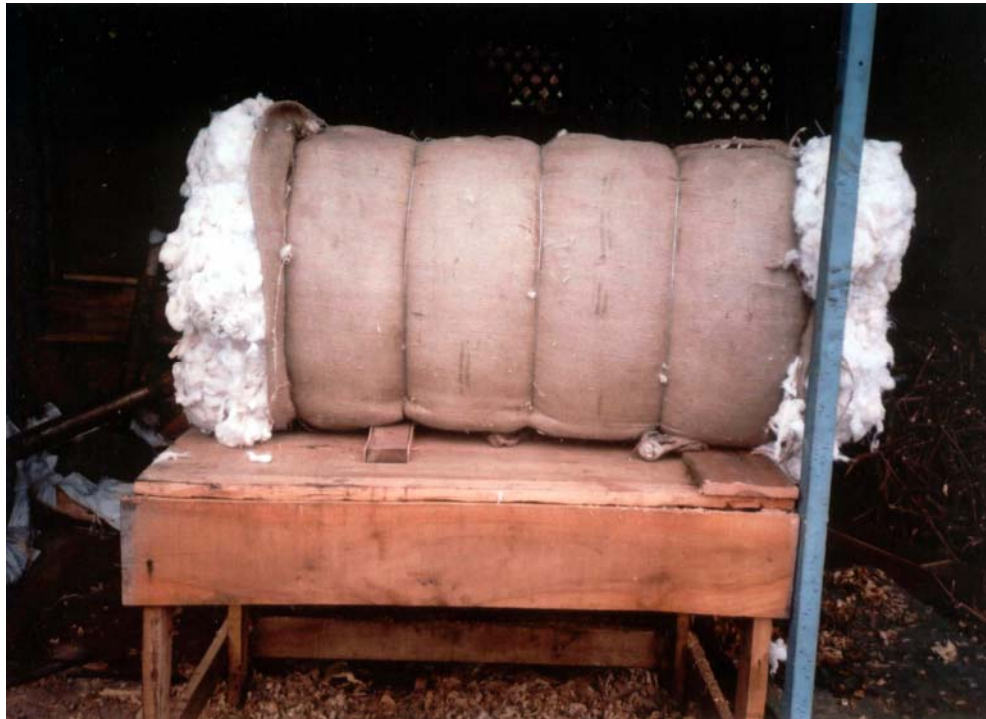
Figure 4 Compressed bale from the mechanical press
