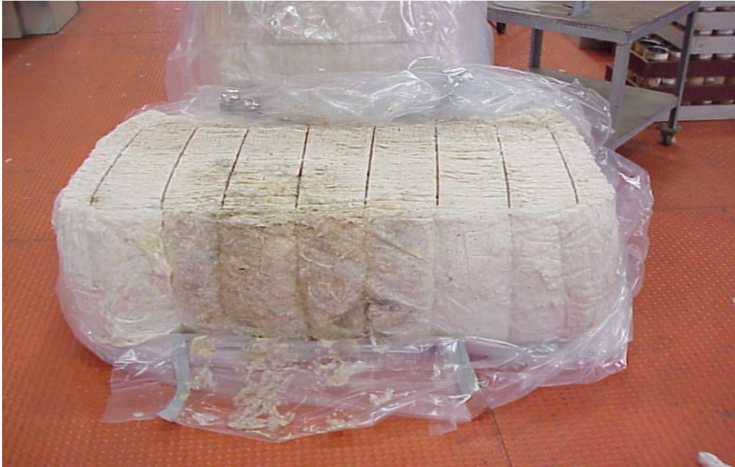
Figure 1. Typical yellow or dark discoloration water damage observed when the polyethylene coverings were removed from the bales where moisture was added.
