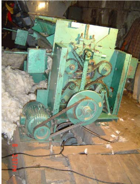
Figure 5 (Left) Modified DR gin showing the improved power transmission system and (Right) the gear train of existing DR gin.
