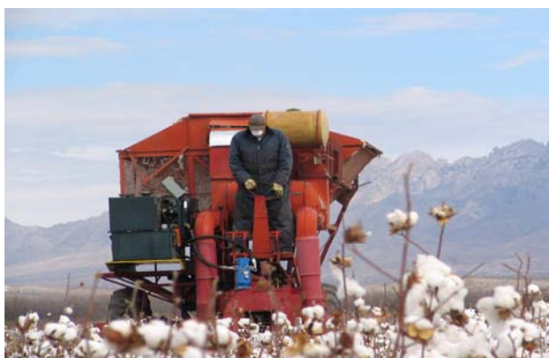
Figure 1. The modified 1-row cotton picker in action. The drive for the spindles was separated from the drum drive. A hydraulic motor (in blue on the picker head) powered the spindles and doffers. A 37 kW (50 hp) diesel-powered hydraulic pump unit (in gray) was added to power the hydraulic motor.
