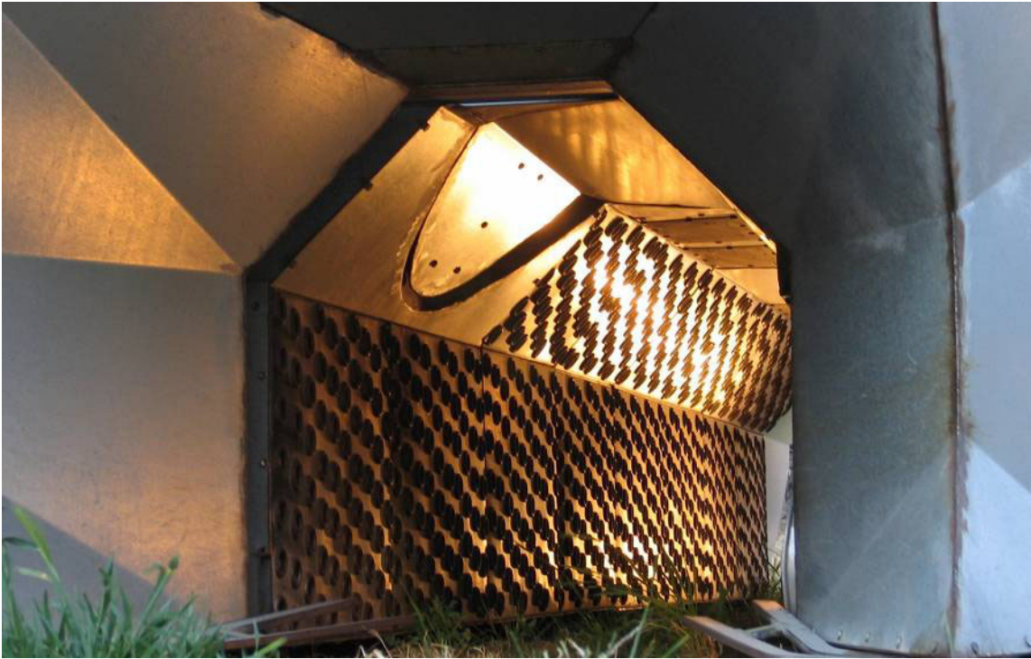
Figure 2. Treatment chamber with nozzles to direct hot air through the cotton canopy.
